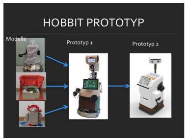
Figure 3.5 The development of HOBBIT robot by TU Wien: first models made by users, then first prototype tested in lab trials, then second prototype tested in homes of older people
