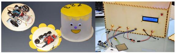
Figure 3.8 The Mattie robot platform. From left to right: first version of the Mattie robot's parts (chassis, touch-to-sound interface, hull), and the sensor box
