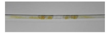
Fig. 2.3: Straw as sample holder with compensation capsules. In the middle a window is cut in the straw to easy change the capsule with the sample in it. The other four capsules are fixed with vanish to the straw.
