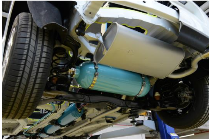
Figure 4- 5: Accumulator placing in the 2013 prototype of the Hybrid Air [16]
