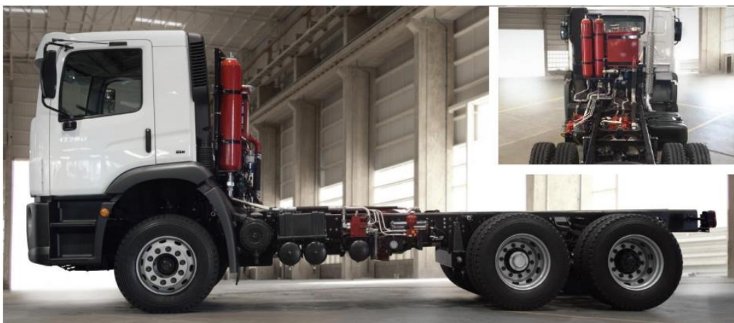
Figure 2- 20: Implementation of the HRB on a truck (red components) [18]
