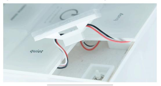
Figure 12: 3D printed button cap with LED wires and Plexiglas cover.
