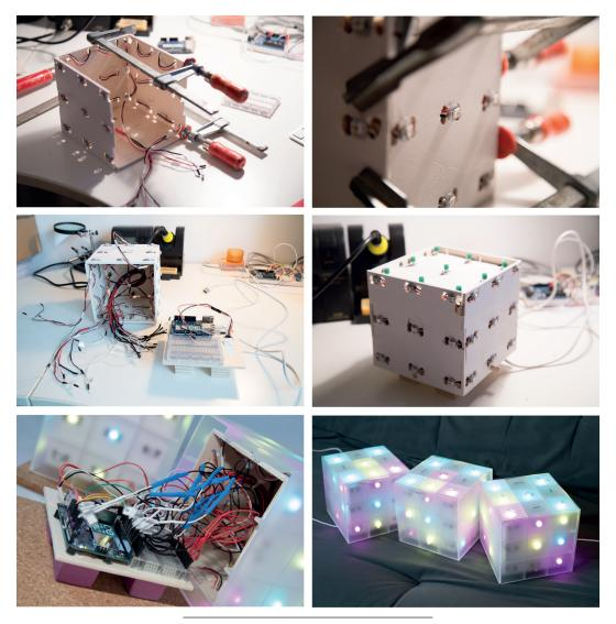
Figure 11: *Awareness cube* construction; a: assembly of wooden sidewalls; b: LEDs mounted on the sidewalls; c: inner cube and bottom plate with microcontroller and breadboard; d: finished inner cube; e: opened cube with transparent Plexiglas shell; f: three completely finished and illuminated *awareness cubes*.
