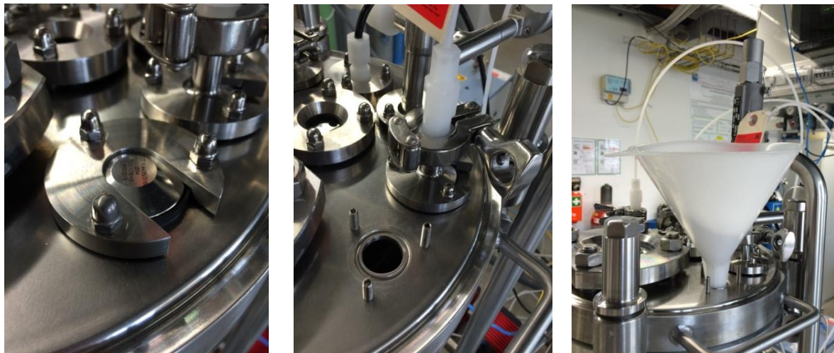
Figure 82: Procedure to Fill the Reactor via the Excess Port on the Lid
