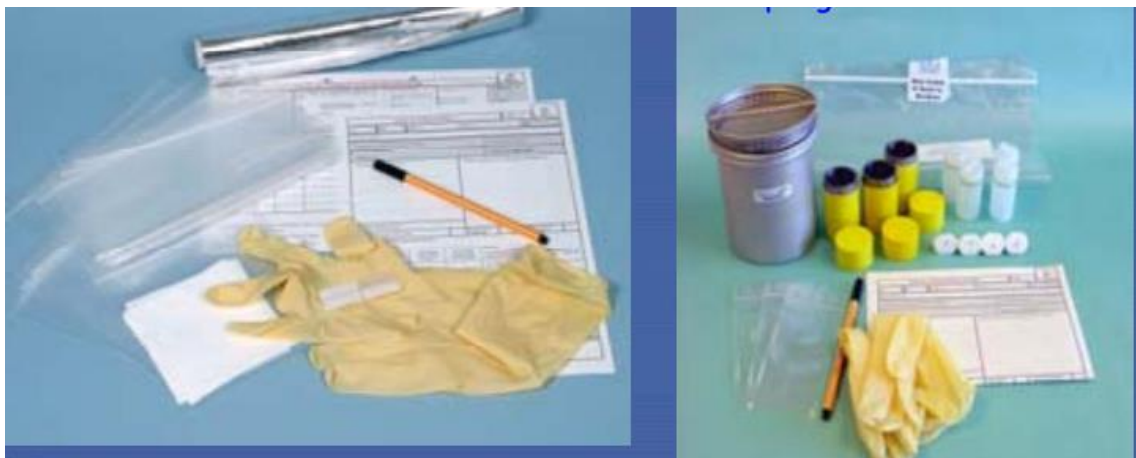
Figure 2.2.1: Standard swipe sample kit used for Environmental Sampling (Source: Penkin 2009)
