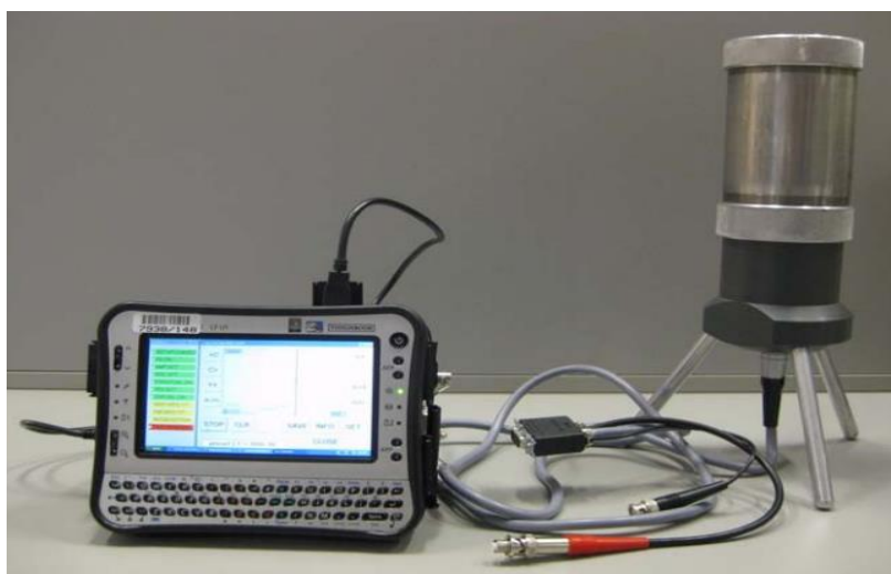
Figure 2.4.2: Miniature Multi Channel Analyser with NaI Detector (Source: IAEA 2011)
