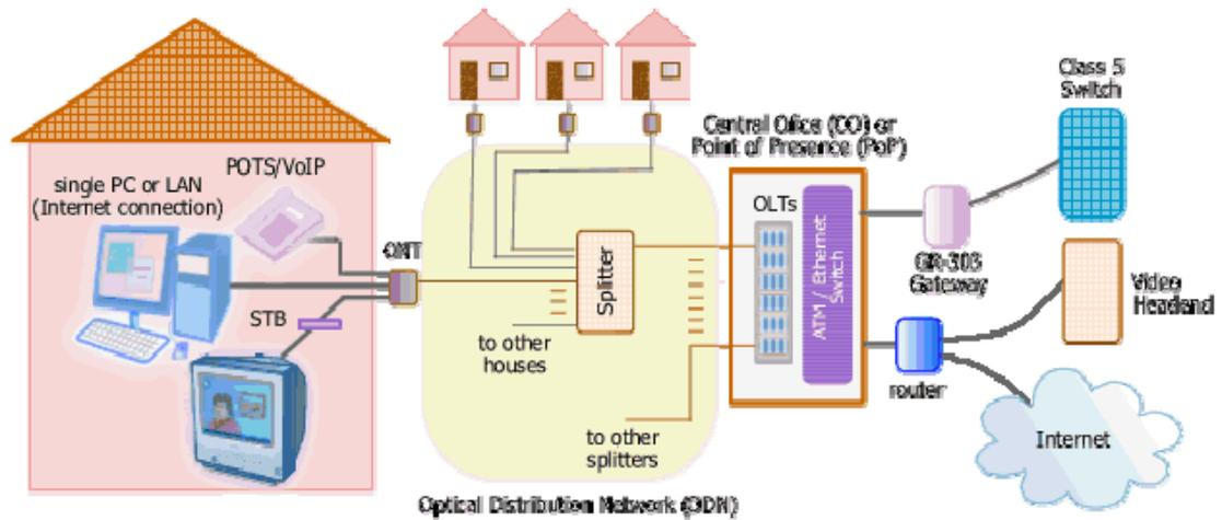
**Figure 5 - Generic fiber to the premises connectivity example (Conniq, 2016)**
