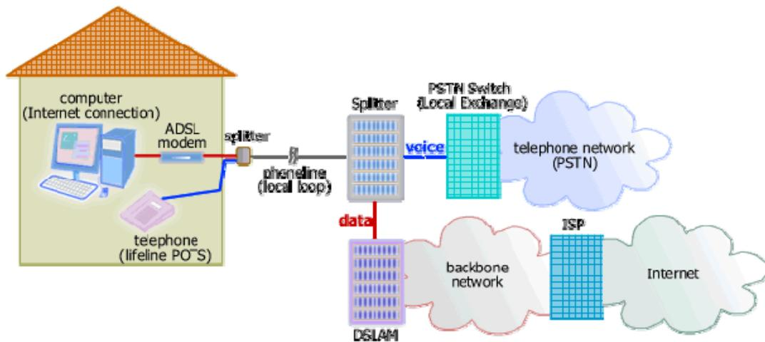
**Figure 3 – Generic DSL connectivity example (Conniq, 2016)**
