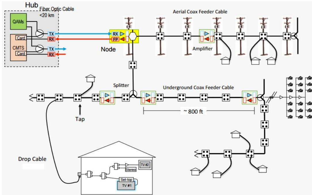
**Figure 14 - HFC underground and aerial installation and its components (Conniq, 2016)**
