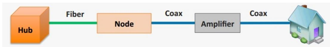
**Figure 13 - HFC HUB to end-customer connectivity**
