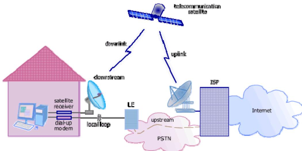
**Figure 7 - Generic satellite connectivity example (Conniq, 2016)**
