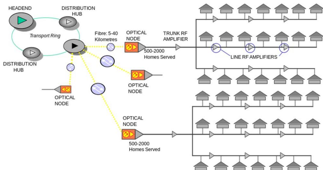
**Figure 9 - Typical HFC network architecture (Wikipedia, 2016)**
