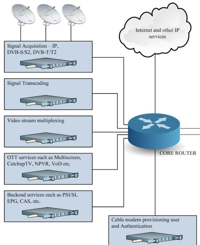
**Figure 11 - Head-end generic connectivity scheme**
