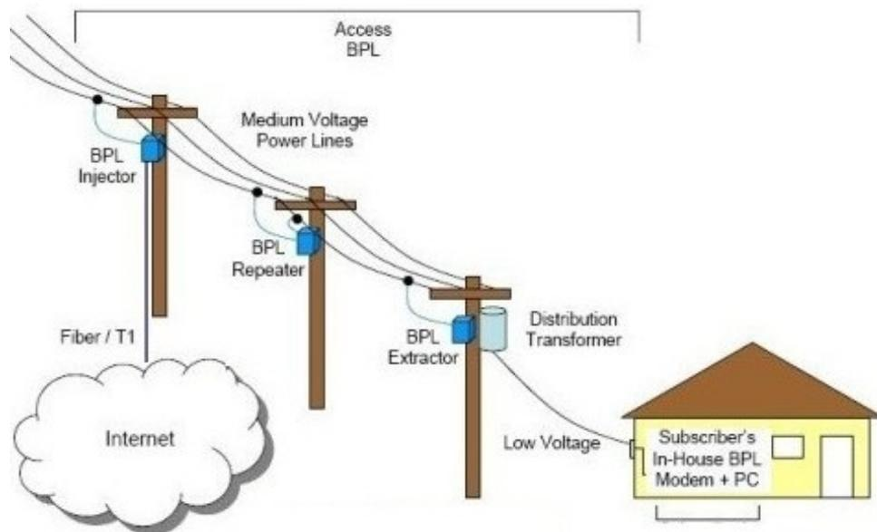
**Figure 8 - Generic broadband over power line connectivity example (Connig, 2016)**
