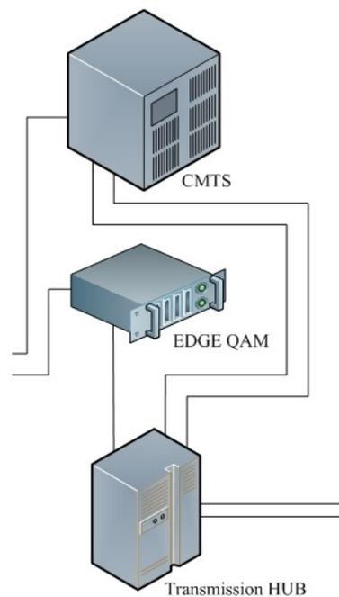
**Figure 12 - HFC generic aggregation/distribution network segment**
