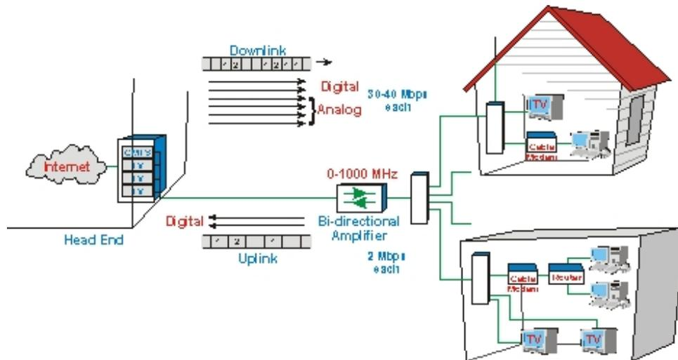
**Figure 4 - Generic cable modem connectivity example (Harte, 2007)**
