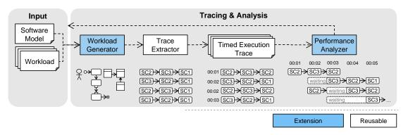
Figure 3.8: Model-Based Performance Analysis Framework
