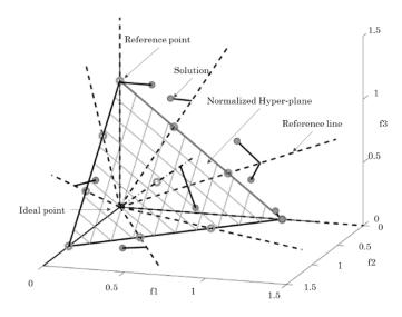
Figure 5.16: Normalized Reference Plane for Three Objectives
