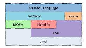
Figure 4.9: Technology Stack of MOMoT
