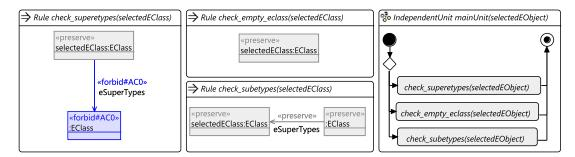
(a) Initial Check for Remove Empty Sub-Class-Refactoring
