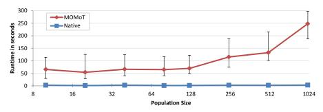
Figure 5.10: Total Runtime Comparison for Stack System: Native Encoding vs MOMoT
