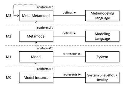
Figure 2.1: Four-Layered Metamodeling Stack (adapted from [BCW12, Küh06])
