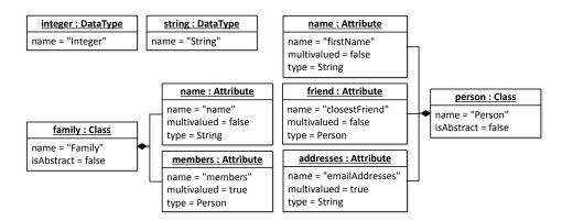
Figure 2.4: Source Model Conforming to the Class Diagram Metamodel
