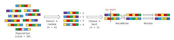
Figure 2.13: Steps Performed by Evolutionary Search Methods in Each Iteration
