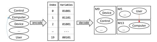
Figure 5.8: Native Encoding for the Modularization Case Study
