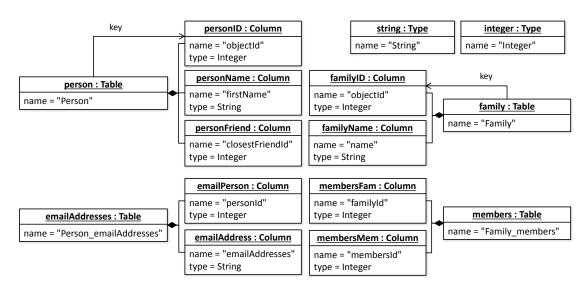
Figure 2.6: Target Model Conforming to the Relational Metamodel
