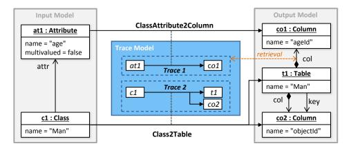
Figure 2.5: Excerpt of the Trace Model Used by ATL During Execution
