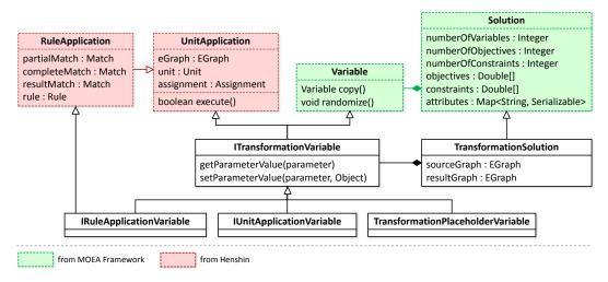
Figure 4.10: Solution Definition in MOMoT
