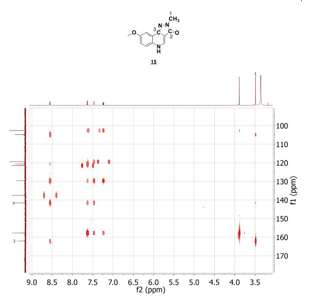
Figure 14 Section of HMBC NMR of 8-methoxy-2-methyl-2,5-dihydro-3H-pyrazolo[4,3-c]quinolin-3-one (15)
