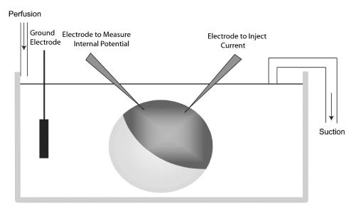
Figure 15 Diagram of the two-electrode voltage clamp<sup>53</sup>
