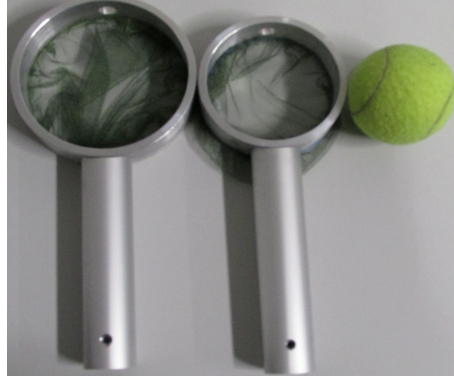
Figure 5.5: Grippers used for ball catching.
