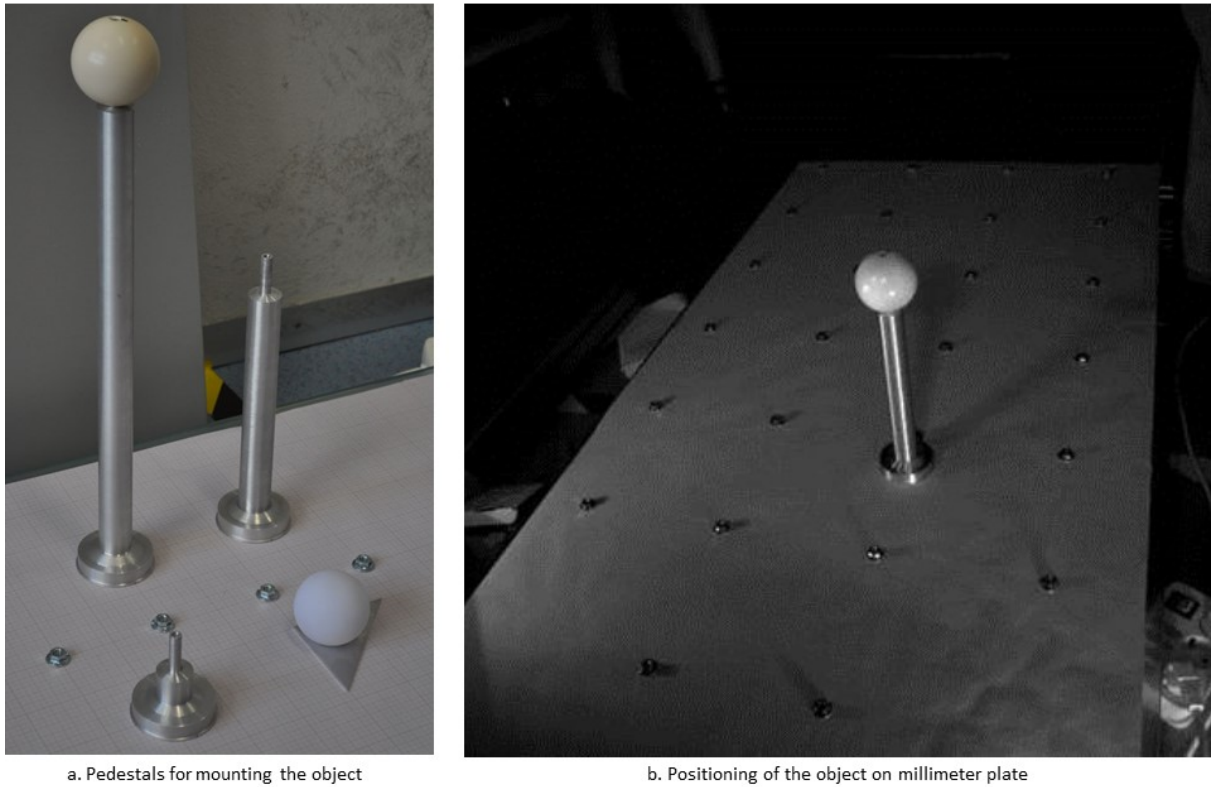
Figure 3.9: The setup for the accurate positioning of the spheres in space. The spherical objects are mounted on the pedestals with precise height (subfigure a). The pedestal in the right bottom corner of figure a. is intended for the self-lighting sphere. Accurate positioning in the vertical dimension is provided by the pedestals while accurate positioning in two horizontal dimensions is provided by the millimeter plate. Subfigure b show an example of accurate object positioning in space: the pedestal is put into specific position on the plate. In other cases the objects on various pedestals were put into various positions.
