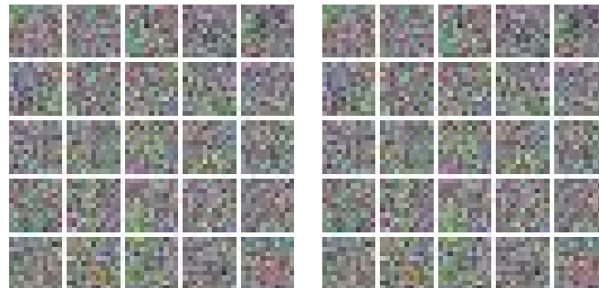
Figure 7.1: Weights before (left) and after (right) training a 2-class model with standard stochastic gradient descent. There is almost no change, showing that the network does not learn features.
