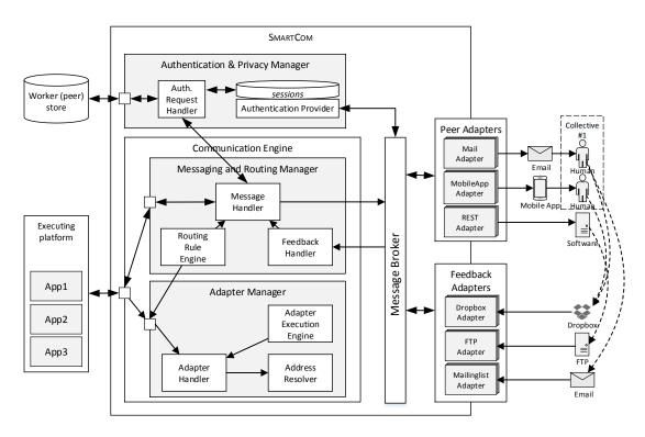
Figure 6.2: Internal architecture of SMARTCOM middleware.
