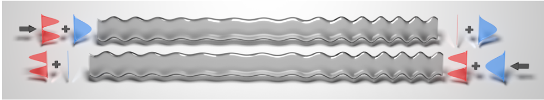
Figure 3.1: Schematic of an asymmetric mode-switch that projects the EP-encircling shown in Fig. 2.2 to a waveguide that strongly attenuates one of its two transverse modes depending on the injection direction. The parameter-space trajectories describing counter-clockwise and clockwise loops around the EP shown in panels a and b of Fig. 2.2 correspond to left and right injection shown here at the top and bottom, respectively.
