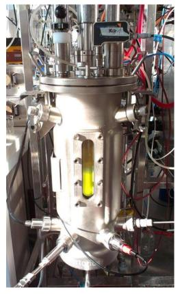
Figure 4: 15 L stainless steel Biostat Cplus bioreactor (Satorius, Göttingen, Germany). Fed batch experiments of this Thesis were conducted in this Fermenter. In this picture an induced *E. coli* culture produces the marker protein enhanced green fluorescent protein.
