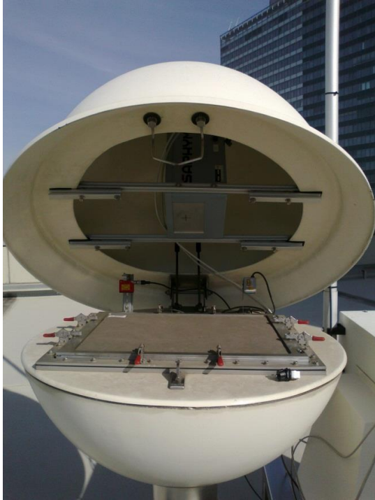
Figure 14 and 15 LaBr detector placement inside the station. If the lid is open the direct placement of the detector above the filter can be seen. (Khrustalev et al., 2015)
