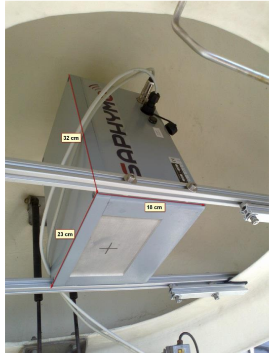
Figure 14 and 15 LaBr detector placement inside the station. If the lid is open the direct placement of the detector above the filter can be seen. (Khrustalev et al., 2015)
