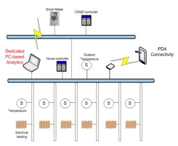
Fig. 8: Overview of systems architecture for field validation as part of an integrated home automation system. Each apartment building has 6 separate apartments.
