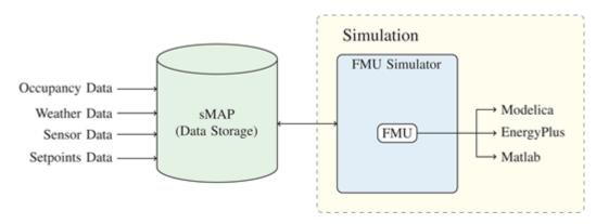
Fig. 11: Online Energy Simulation Architecture (Mattera et.al 2018)
