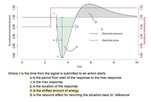
Fig. 1: Potential of energy flexibility as a function of a building's or system's response to a step change in the external penalty signal (Jensen et al. 2017).
