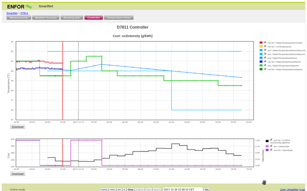
Fig. 6: A house (D7811) using CO 2 -based control. This minimizes the total CO 2 emission related to heating up the swimming pool.
