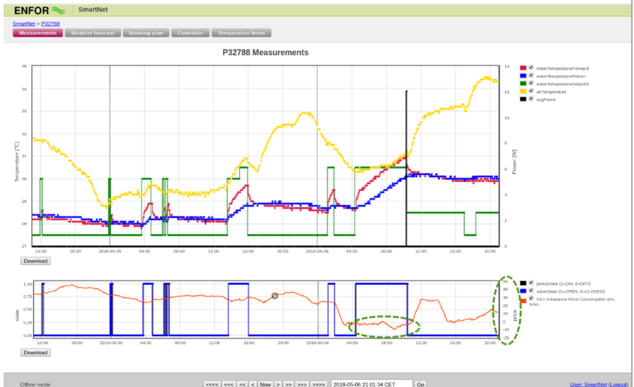
Fig. 7: A house (D32788) using price-based control. This minimizes the total costs related to heating up the swimming pool. This screen plot contains a period with negative power prices (green ellipsoid).
