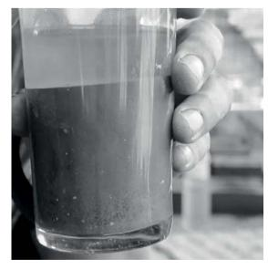
fig. 19: Result of the sedimentation test carried out on the site of Afarkindergarten-project
