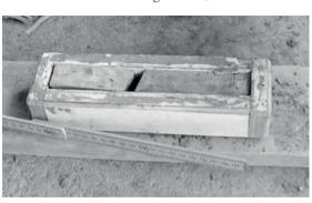
fig. 22: Linear shrinkage test carried out on the site of Afarkindergarten-project
