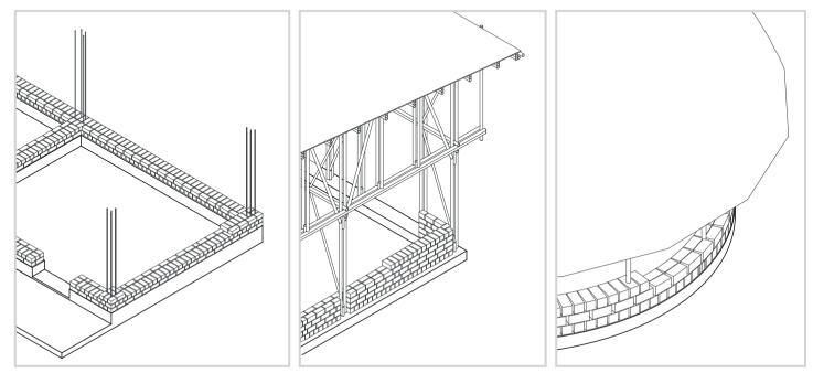
fig. 211: Brickwork of AK-project M 1:100
