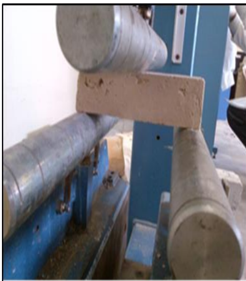
Figure 4-10 Flexural bending test on clay prisms
