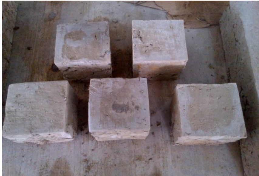
Figure 4-6 Prepared clay specimens for the compression test
