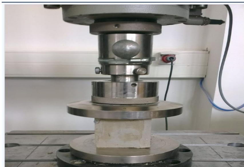
Figure 4-7 Compression test carried out on the prepared clay specimens
