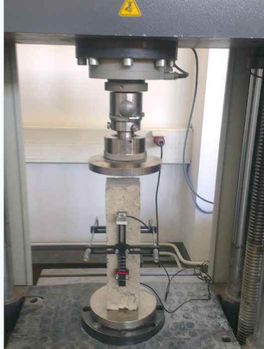
Figure 4-17 Test setup for determining the elasticity modulus
