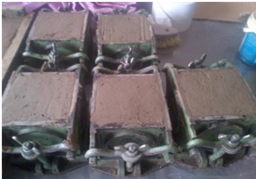
Figure 4-5 Prepared clay in the formwork for the compression test
