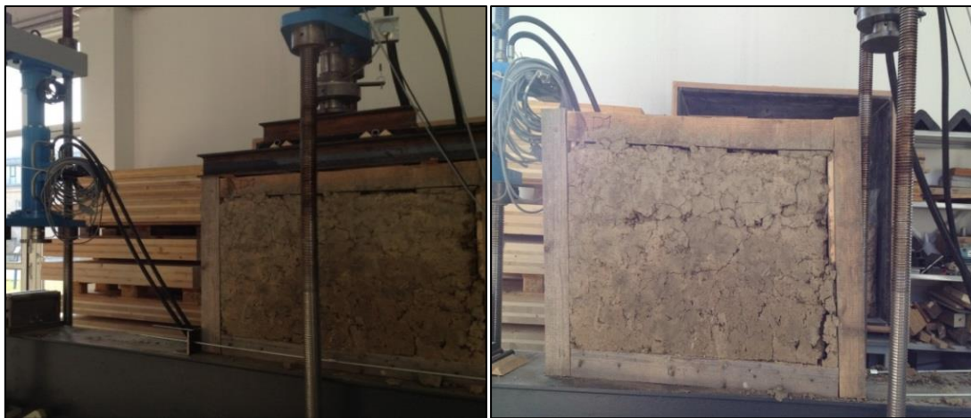
Figure 4-32 Shear strength test for wall section D1
