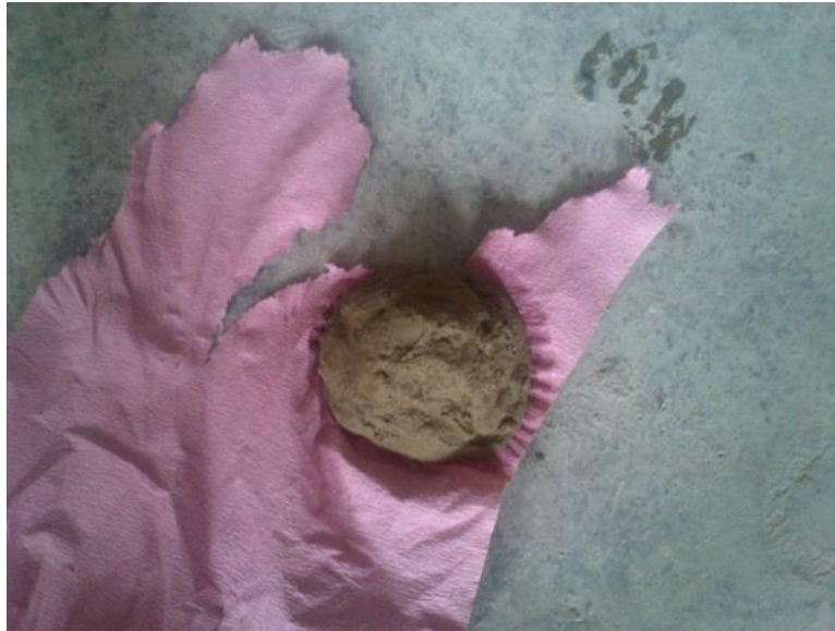
Figure 4-4 Slump test for prepared clay
