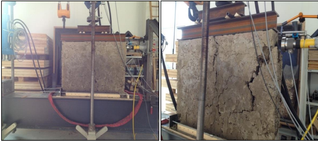
Figure 4-29 Shear strength test for wall section C2
