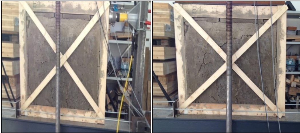
Figure 4-35 Shear strength test for wall section E1
