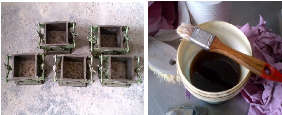
Figure 4-3 formwork preparation for the compression test
