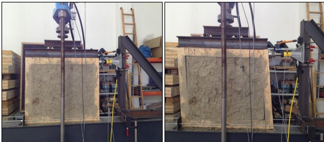
Figure 4-24 Shear strength test for wall section B1
