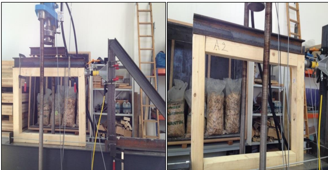
Figure 4-21 Shear strength test for wood frame A1 and A2
