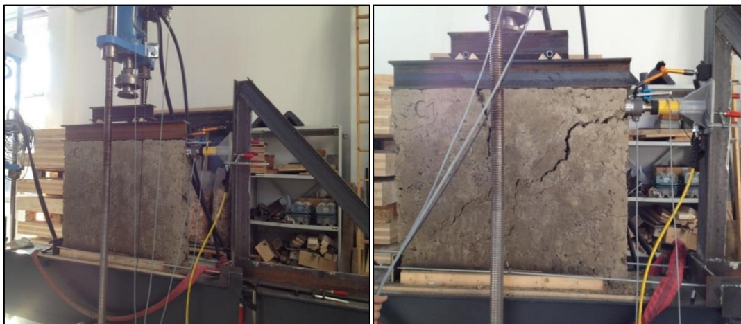
Figure 4-28 Shear strength test for wall section C1
