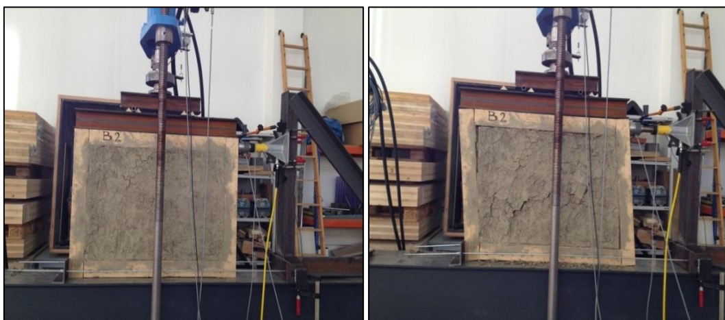
Figure 4-25 Shear strength test for wall section B2
