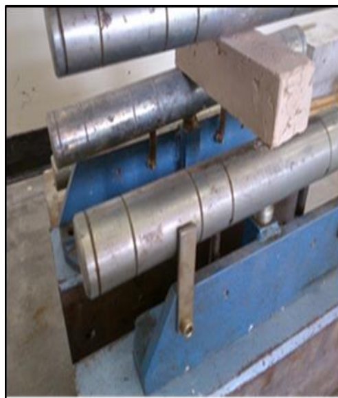
Figure 4-10 Flexural bending test on clay prisms
