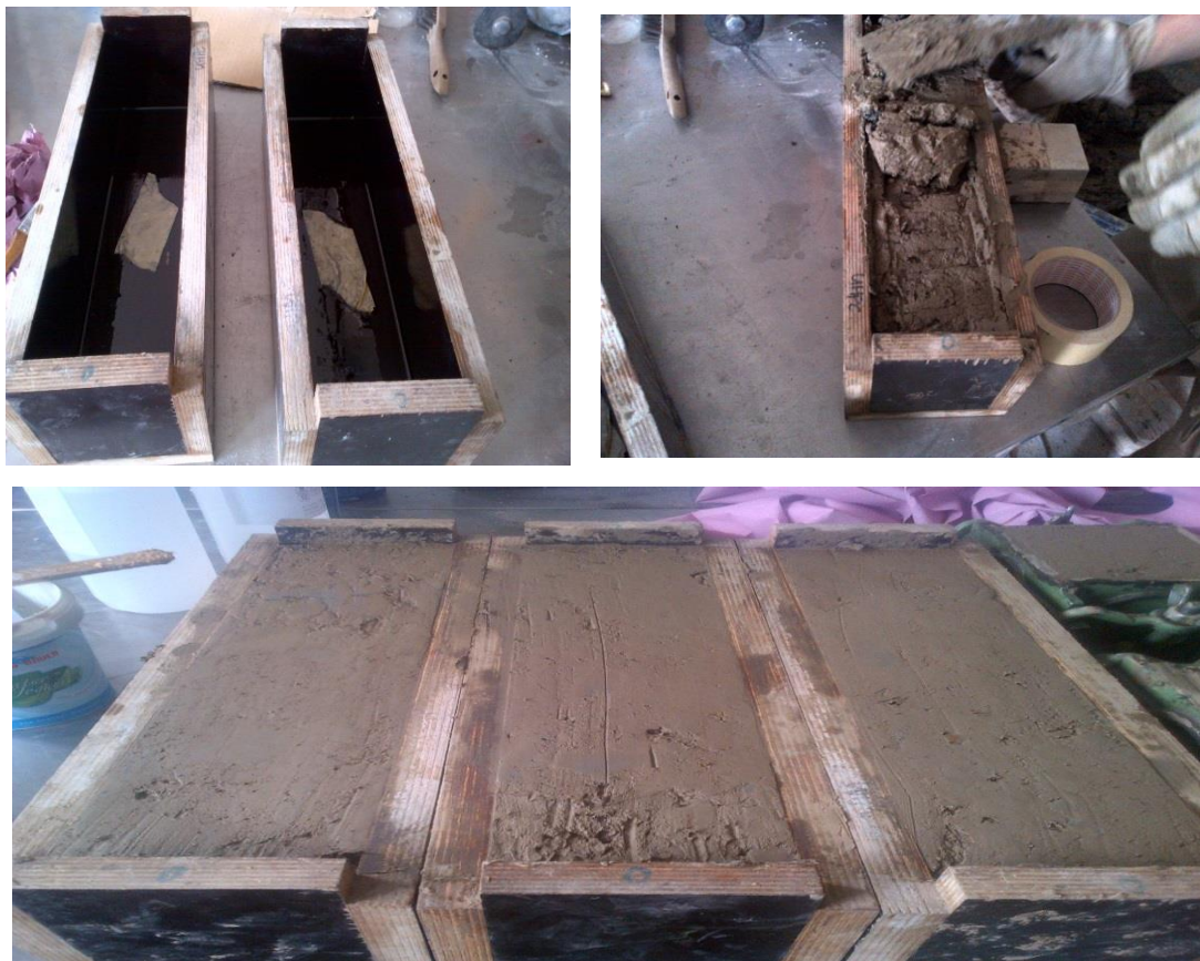
Figure 4-16 Preparation of clay prisms for the elasticity modulus test
