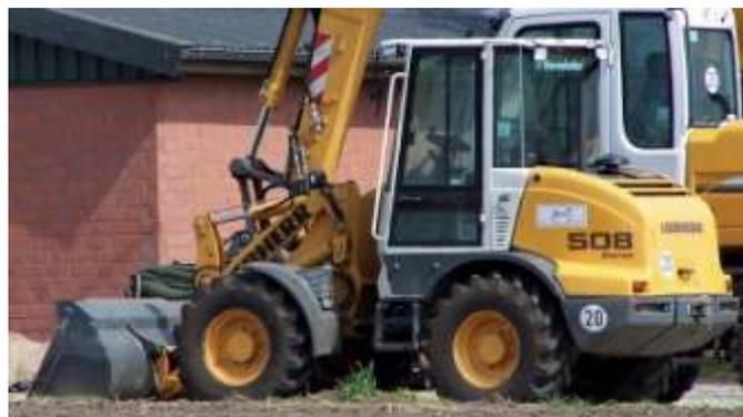
Abb. 55 Radlader Liebherr L 508 Stereo
