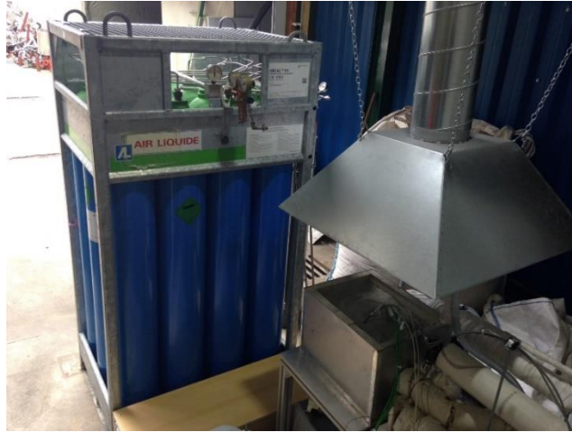
Figure 24 Reformer under the aspiration system and forming gas bundle
