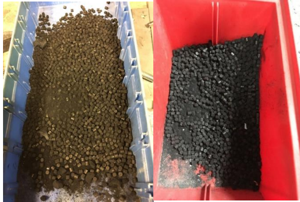
Figure 28 Ruined Ni-catalysts during the change (left: first catalyst, right second catalyst).
