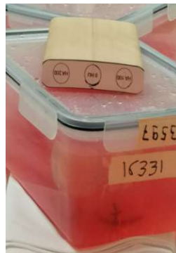
Figure 2.4: Samples submerged in saline solution for the QCT scan, including the phantom on top of the box
