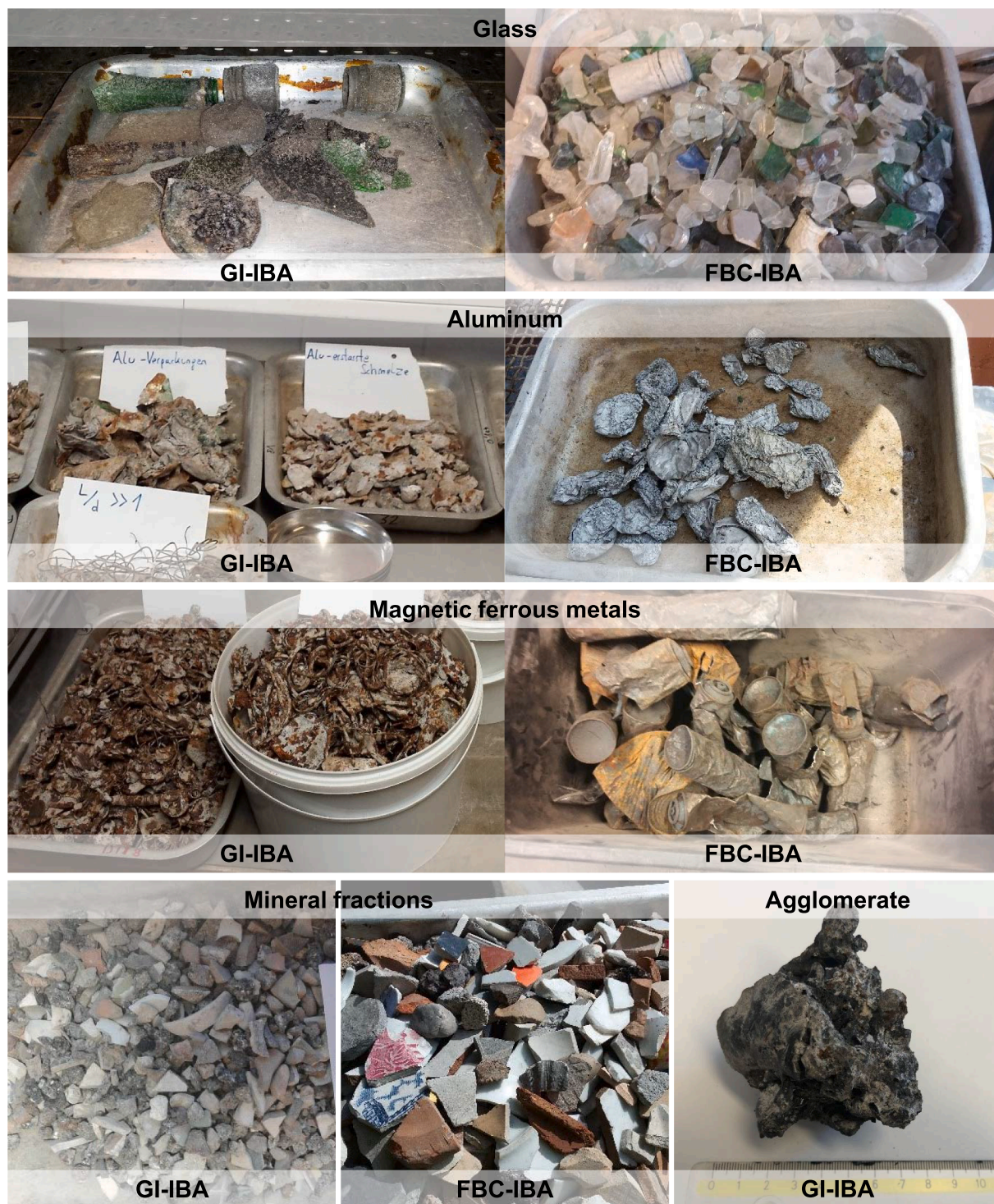
Fig. 4. Glass (1st row), aluminum (2nd row), and magnetic ferrous metals (3rd row) fractions of IBA from GI (left) and FBC (right). 4th row: Mineral fractions of IBA from GI (left) and FBC (middle). Agglomerate of glass, metals and mineral phases in GI-IBA (right).
