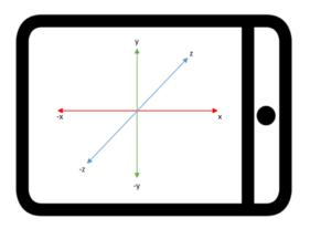
Figure 5.7: The accelerometer makes it possible to get values for the linear acceleration.
