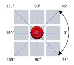
Figure 5.3: Determining the swipe direction of the user input.
