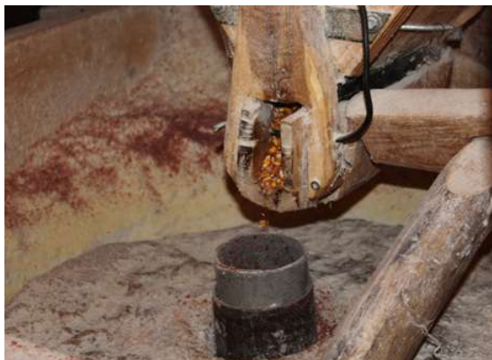
Fig. 118 Close- up image of the grinding mechanism during grinding process, at the Mill of Bekim Binak Kamberaj , Uqë, Istog
