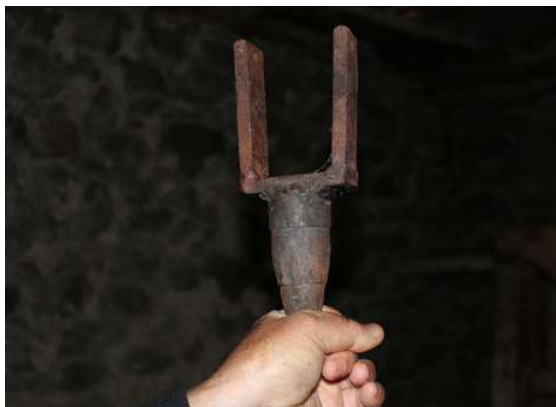
Fig. 119 Metallic part of the stone spindle at the Mill of Sallaj Family, Junik
