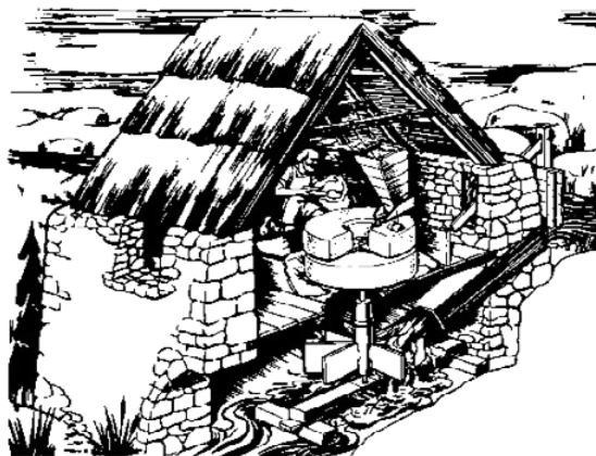
Fig. 7 (left) Horizontal mill, Norse Mill: reconstruction based on a post-medieval example
