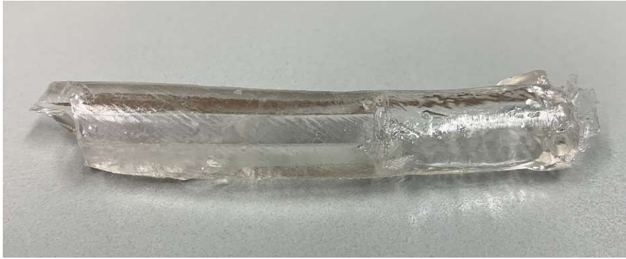
Figure 3.21: A demolded silicon tube. The ends are fringed and the tube is not complete.
