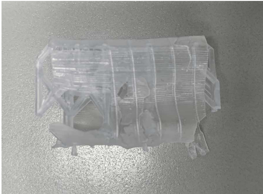
Figure 3.12: The cylinder collapsed after printing, due to too thick wall thickness.
