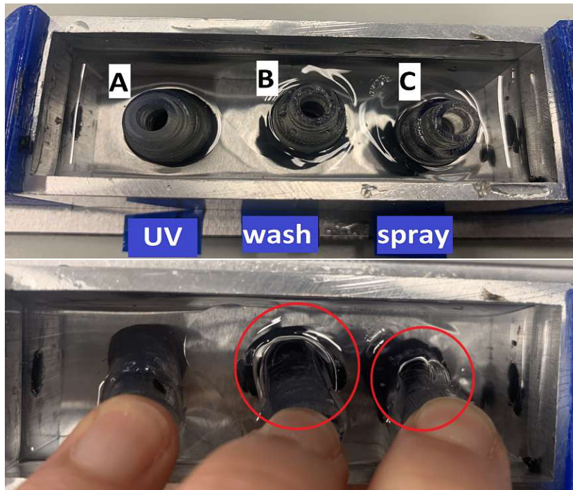
Figure 3.24: Printed connector in silicon after using different methods of post processing. upper image: A - part was placed in the UV chamber. B - part was washed. C - part was sprayed with clear lack. bottom image: The red circles mark a gap between silicon and tube.
