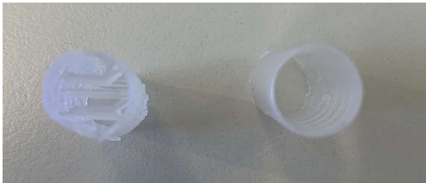
Figure 3.13: Two different cylinders with different support system. The left cylinder was printed with inner support structures, while there were only used support structures on the outside for the right cylinder.
