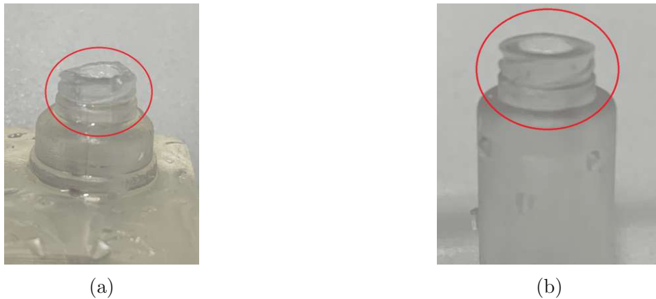
Figure 3.6: A slightly damaged Luer connector (a) and a Luer connector with no damage from post processing (b).
