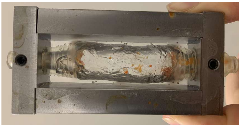
Figure 3.28: The silicon form after the form was filled with silicon and put into an UV chamber.
