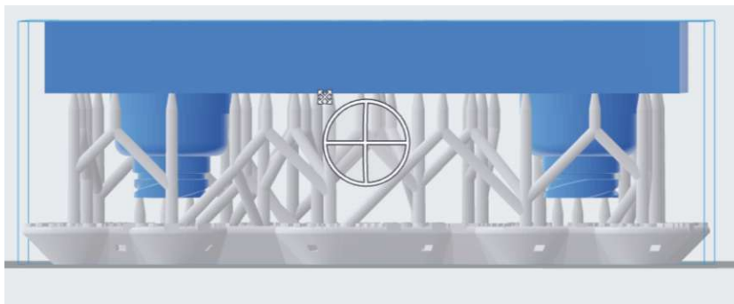
Figure 3.5: Close up of a channel in the printing interface. The blue part is the channel and the light grey mesh shows the needed support structure. The white circle in the middle is a tool to move the component.
