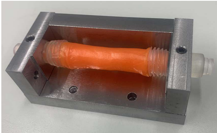
Figure 3.27: The silicon form with the shaped wax cylinder, in orange, merged together.
