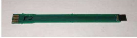
(b) PCB chip carrier with sensorchip bonded to its tip.
