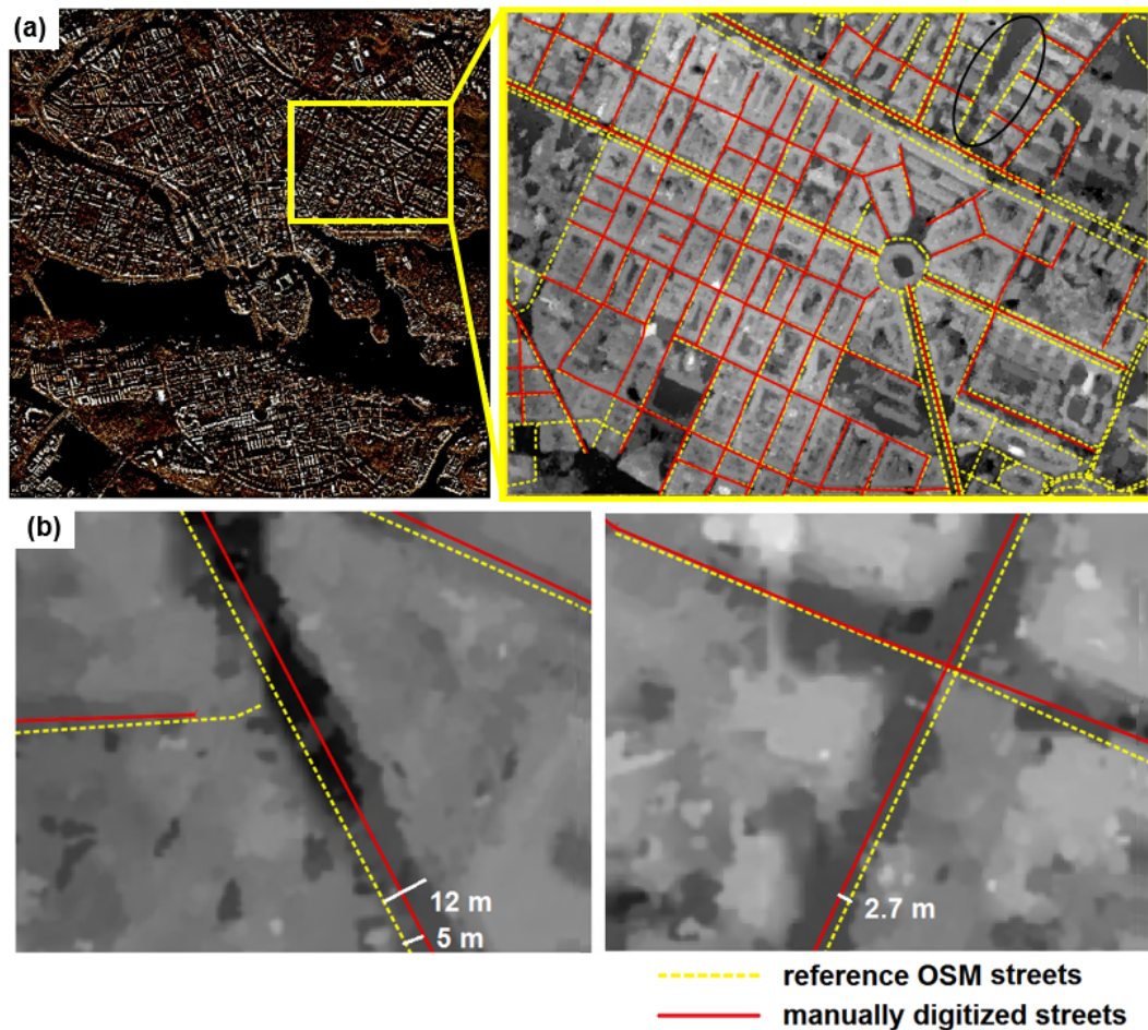
Figure 4.16: DSM Stockholm geolocation: (a) orthophoto with marked area of interest and zoom-in in the DSM with OSM-reference and manually digitized street axes; (b) offset in planimetry.
